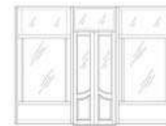
Figure 7.33.17 All glass windows and doors with modern designs are not an acceptable option.
